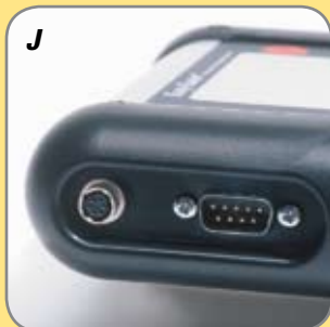
Countersunk connectors, well protected against external damage.
